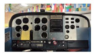
...and then it is sent out for powder coating and the bottom panel is sent out to be CNC cut and laser etched.
